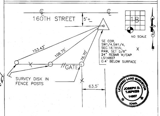
PREVIOUSLY RECORDED IN BOOK 1999, PAGE 3217 MONUMENT DESCRIPTION AND HOW ESTABLISHED HALL&HALL PIN&CAP W/TIES DESTROYED DURING COUNTY ROAD CONSTRUCTION, REPLACED WITH 5/8"X24" REBAR AND LS CAP 14807 0.4' BELOW ROAD SURFACE PER HALL&HALL ACQUISITION PLAT PARCEL NO. 98-106
