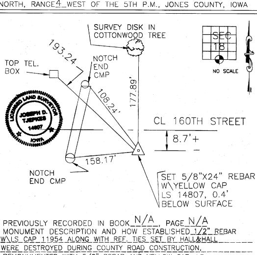
W\LS CAP 11954 ALONG WITH REF. TIES SET BY HALL&HALL WERE DESTROYED DURING COUNTY ROAD CONSTRUCTION, REMONUMENTED WITH 5/8" REBAR AND YELLOW CAP, LS
