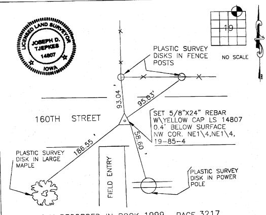
PREVIOUSLY RECORDED IN BOOK 1999, PAGE 3217 MONUMENT DESCRIPTION AND HOW ESTABLISHED HALL&HALL PIN CAP AND REFERENCE TIES DESTROYED DURING COUNTY ROAD CONSTRUCTION, REMONUMENTED CORNER WITH 5/8"X 24" REBAR WITH YELOLW CAP LS 14807 0.4' BELOW SURFACE PER HALL&HALL ACQUISITION PLAT (PARCEL NO. 98154) AND SET NEW REFERENCE TIES
