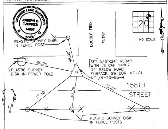
PREVIOUSLY RECORDED IN BOOK 1999, PAGE 3221 MONUMENT DESCRIPTION AND HOW ESTABLISHED HALL&HALL PIN&CAP AND REFERENCE TIES DESTROYED DURING ROAD CONSTRUCTION, REMOMUMENTED WITH 5/8"X24" REBAR WITH YELLOW CAP LS14807 (PER HALL &HALL ACQUISITION PLAT [PARCEL NO. 98-114]) 0.4' BELOW ROAD SURFACE. SET NEW REFERENCE TIES AS INDICATED ABOVE.
