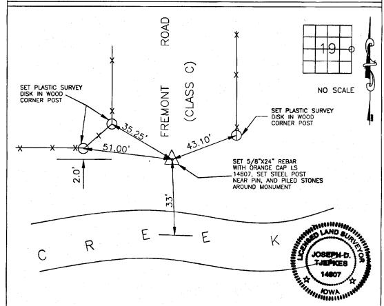
PREVIOUSLY RECORDED IN BOOK N/A , PAGE N/A MONUMENT DESCRIPTION AND HOW ESTABLISHED SET 5/8"X24" REBAR WITH ORANGE CAP LS 14807 ON LINE AND ON SPLIT BETWEEN NORTHEAST CORNER SECTION 19 AND THE SOUTHEAST CORNER OF SECTION 19.
