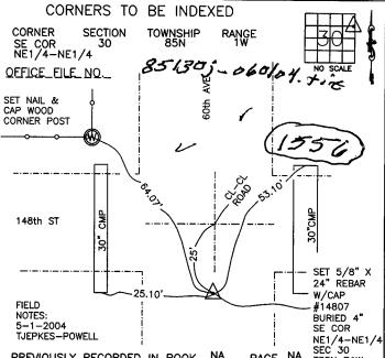
PREVIOUSLY RECORDED IN BOOK NA , PAGE NA T85N R1W MONUMENT DESCRIPTION AND HOW ESTABLISHED PER BREAKDOWN OF SECTION 30 T85N R1W, SET 5/8"X 24" REBAR W/YELLOW CAP #14807 ON LINE AND MIDWAY BETWEEN E 1/4 & NE COR. SECTION 30. TOP OF REBAR BURIED 4" IN ROADBED. TIES AS INDICATED FOR SE COR. NE1/4-NE1/4 SECTION 30 T85N R1W.
