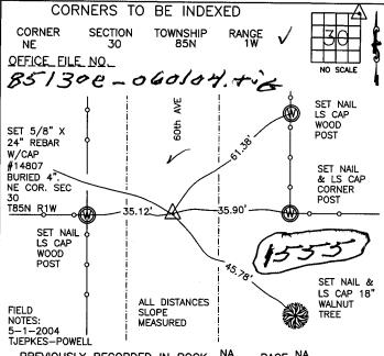
PREVIOUSLY RECORDED IN BOOK NA , PAGE NA MONUMENT DESCRIPTION AND HOW ESTABLISHED PER PHYSCIAL EVIDENCE AT CENTER LINE OF ROAD AND FENCE LINES RUNNING EAST & WEST, SET 5/8"X 24" REBAR W/YELLOW CAP # 14807 BURIED 4". TIES AS INDICATED FOR NE CORNER SECTION 30 T85N R1W.
