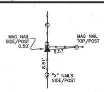
S 1/4 CORNER SECTION 8, T84N, R4W FD. 1/2" REBAR W/YELLOW CAP NO. 8165
