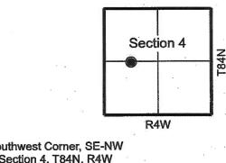
Southwest Corner, SE-NW Section 4, T84N, R4W Found 5/8"dia rebar w/cap 0.3' above ground
