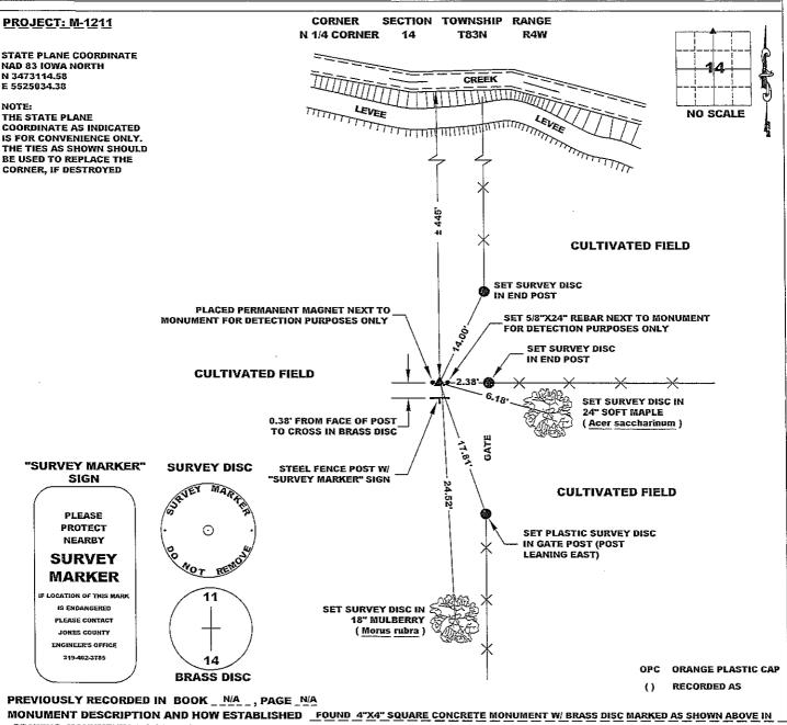
DRAWING. MONUMENT WAS 9" BELOW EXISTING GROUND SURFACE. MONUMENT HAS NO MAGNETIC SIGNATURE THAT CAN BE DETECTED. PLACED 5/8"X24" REBAR AGAINST THE EAST FACE AND SLIGHTLY BELOW THE SURFACE OF THE MONUMENT AND FURTHER SET WAS A PERMANENT MAGNET NEXT TO THE WEST FACE AND SLIGHTLY BELOW THE SURFACE OF THE MONUMENT. A STEEL FENCE POST WITH A YELLOW "SURVEY MARKER" SIGN ATTACHED WAS SET 0.38' SOUTH OF MONUMENT'S CENTER TO BEAR WITNESS TO THE CORNER.
