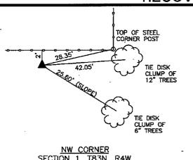
NW CORNER SECTION 1, T83N, R4W FD. 5/8" REBAR (OVER 24" DEEP STONE)
