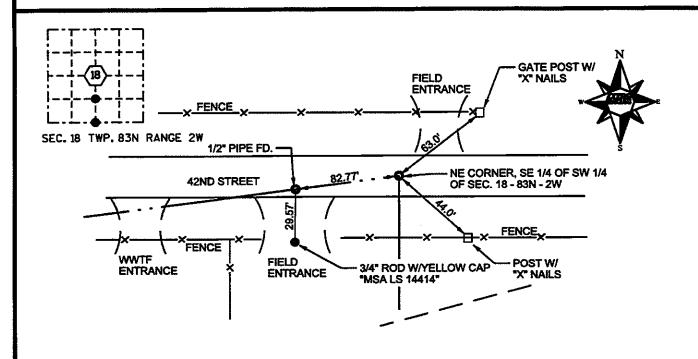
NE CORNER OF SE 1/4 OF SW 1/4 OF SECTION 18 - T83N - R2W
