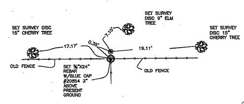
PREVIOUSLY RECORDED IN BOOK NA PAGE NA MONUMENT DESCRIPTION AND HOW ESTABLISHED SET %"X24" REBAR WITH BLUE CAP #20854 AT OLD FENCE CORNER SPLIT. FOUND ¾" IRON ROD STICKING OUT OF THE TOP OF CORNER POST. OLD FENCE LINES SOUTH, EAST, & WEST. BEST EVIDENCE OF CORNER. TIES AS INDICATED.
