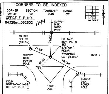
PREVIOUSLY RECORDED IN BOOK. NA , PAGE NA MONUMENT DESCRIPTION AND HOW ESTABLISHED FD.5/8" IRON PIN AT CENTER SEC.28 T84N R3W ON CENTERLINE ROAD 165th AVE. & 80th ST. 24" BELOW PRESENT ROAD SURFACE, PER ROAD RECORDS IN JONES COUNTY ENGINEER'S OFFICE. SET 5/8"X24" REBAR W/ORANGE CAP #14807 ON TOP OF ORIGINAL PIN, AT CENTER OF SECTION 28 T84N R3W. TIED AS INDICATED.
