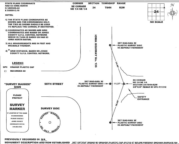
MONUMENT DESCRIPTION AND HOW ESTABLISHED SET 5/8"X24" REBAR W/ ORANGE PLASTIC CAP #11310 6" BELOW PRESENT GROUND SURFACE ON A SAFETY ENTRANCE ON THE EAST SIDE OF IOWA HIGHWAY No. 136 OPPOSITE INTERSECTION WITH 98TH STREET. CORNER WAS SET EQUIDISTANT AND ON LINE BETWEEN THE NE CORNER OF SECTION 24-T84N-R2W (REFER TO BOOK 356, PAGE 97) AND THE E 1/4 CORNER OF SAID SECTION 24 (REFER TO RECORDER'S **DOCUMENT 2005 2259).**
