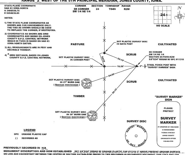
MONUMENT DESCRIPTION AND HOW ESTABLISHED SET 5/8"X24" REBAR W/ ORANGE PLASTIC CAP #11310 3" ABOVE PRESENT GROUND SURFACE
