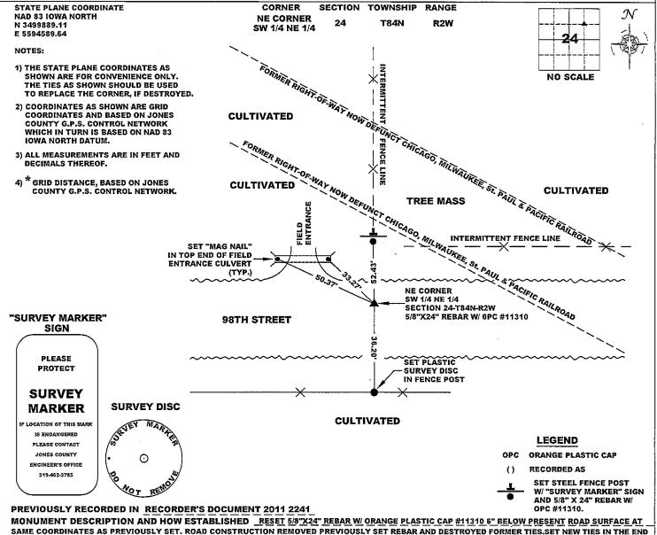
MONUMENT DESCRIPTION AND HOW ESTABLISHED RESET 5/8"X24" REBAR W/ ORANGE PLASTIC CAP #11310 6" BELOW PRESENT ROAD SURFACE AT SAME COORDINATES AS PREVIOUSLY SET. ROAD CONSTRUCTION REMOVED PREVIOUSLY SET REBAR AND DESTROYED FORMER TIES.SET NEW TIES IN THE END OF A NEWLY EMPLACED FIELD ENTRANCE CULVERT AND SET STEEL FENCE POST WITH "SURVEY MARKER" SIGN WITH A 5/8" X 54" REBAR WITH AN ORANGE PLASTIC CAP #11310.
