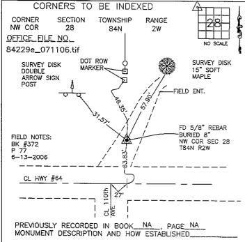
PER TIES ON FILE AT JONES COUNTY ENGINEER'S OFFICE, FILED BY LS#8165 (MEISNER) IN 1992, FOUND 5/8" REBAR BURIED 8". RETIED AS INDICATED. NW CORNER SECTION 28 T84N R2W.
