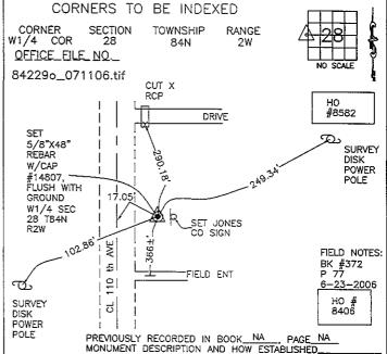
SET 5/8"X48" REBAR W/CAP #14807 IN EAST ROAD DITCH ON LINE BETWEEN FD NW CORNER AND FD SW CORNER SECTION 28 AND ON LINE EAST FROM PLAT OF SURVEY RECORDED AT JONES COUNTY RECORDER'S OFFICE BK I PAGE 8, FILED BY LS#6581 (DILLON). TIES AS INDICATED FOR W1/4 CORNER SECTION 28 T84N R2W.
