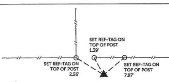
NW CORNER SW 1/4 - NW 1/4 SET 1/2" REBAR 1' SOUTH OF FENCE
