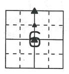
CUT 'X' IN TOP OF CONCRETE CULVERT SET MAG NAIL 90.42. COUNTY CORNER SE1/4, NW1/4, SEC.6, T83N, R1W SET 1/2" REBAR W/ YELLOW CAP SET MAG 58 25
