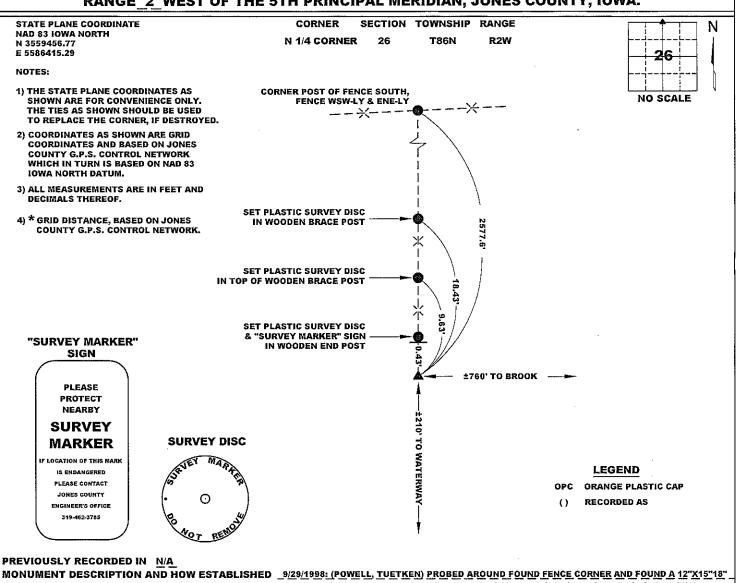
RED GRANITE STONE ON SOUTH SIDE OF NEW CORNER POST 4" ABOVE (THEN) GROUND SURFACE. SET 5/8"X24" REBAR ON NORTH SIDE OF STONE BESIDE CORNER POST. NOTE: AT THAT TIME, AN EAST-WEST EXISTED AS WELL AS THE FENCE TO THE NORTH. CORNER CERTIFICATE WASN'T FILED AT THIS TIME AS THERE WAS NO LAND SURVEYOR ON STAFF.
