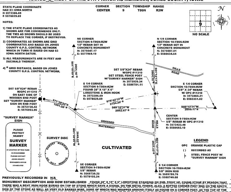
SIDE OF THE STONE AS WELL AS VERY OLD BARBED WIRE, SOME OF WHICH WAS WRAPPED AROUND ITSELF AS FOUND ON A CORNER POST. AS THE TOP OF THE STONE WAS ONLY 10" DEEP, WE LOWERED STONE TO DEPTH OF 26". WE SET A 5/8" X 48" REBAR WITH A PERMANENT MAGNET WRAPPED ONTO THE REBAR BY THE SOUTH SIDE OF THE STONE, AND WE STRAIGHTENED THE IRON HOOK AND PLACED IT ON THE NORTH SIDE OF THE STONE FOR ADDED DETECTION
