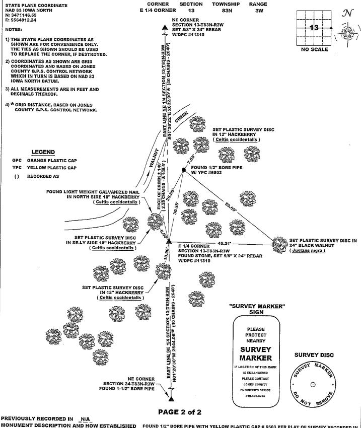
MONUMENT DESCRIPTION AND HOW ESTABLISHED FOUND 1/2" BORE PIPE WITH YELLOW PLASTIC CAP # 6503 PER PLAT OF SURVEY RECORDED IN RECORDER'S DOCUMENTS 2009 1028 AND 2003 1561. FOUND STONE, SET 5/8" REBAR WITH ORANGE PLASTIC CAP #11310 BESIDE STONE. SET STEEL FENCE POST WITH "SURVEY MARKER" SIGN 0.3' NORTH OF 1/2" BORE PIPE AND SET SAME SOUTH OF STONE/REBAR AS WITNESSES TO MONUMENTS . PLEASE REFER TO PAGE 1 OF 2 FOR MORE INFORMATION.
