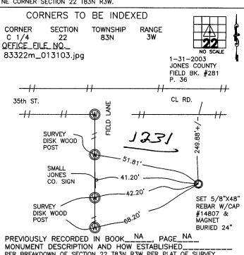
PREVIOUSLY RECORDED IN BOOK NA PAGE NA MONUMENT DESCRIPTION AND HOW ESTABLISHED PER BREAKDOWN OF SECTION 22 T83N R3W PER PLAT OF SURVEY PARCEL #2002-120, SET 5/8'X48" REBAR W/CAP #14807 & MAGNET BURIED 24" IN CULTIVATED FIELD.
