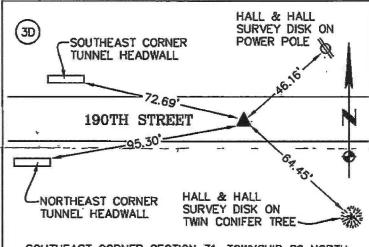
SOUTHEAST CORNER SECTION 31, TOWNSHIP 86 NORTH, RANGE 2 WEST OF THE FIFTH PRINCIPAL MERIDIAN, FOUND 5/8" REBAR FLUSH WITH SURFACE IN CENTERLINE OF ROAD PER PREVIOUS CERTIFICATE DOCUMENT NO. 2005 4303
