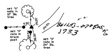
SE CORNER NE-NE SEC. 15 T.86N, R.I.W. OF THE 5TH P.M. PLACED 5/8" STEEL REROD W/ORANGE PLASTIC CAP MARKED "WEBER PLS 15084"
