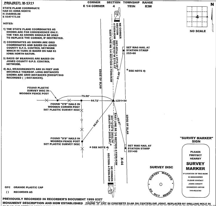
IN SLAB AND SETTING 5/8"X24" REBAR WITH ORANGE PLASTIC CAP #11310 COUNTER SUNK BELOW PAVEMENT SURFACE. FIELD BOOK MISC. 2009-2010, PAGE 149. DATE OF SURVEY: 11/9/10
