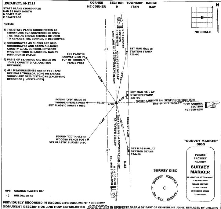
MONUMENT DESCRIPTION AND HOW ESTABLISHED FOUND 'X" CUT IN CONCRETE SLAB 4.36' EAST OF CENTERLINE JOINT, REPLACED BY DRILLING HOLE IN SLAB AND SETTING 5/8"X24" REBAR WITH ORANGE PLASTIC CAP #11310 COUNTER SUNK SLIGHTLY BELOW PAVEMENT SURFACE.
