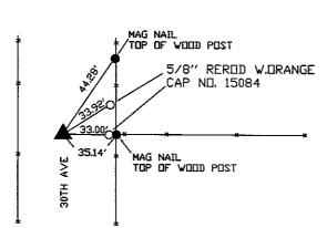
SW COR. NW-SW, SEC. 14, T.84N. R.1W. OF THE 5TH P.M. PLACED 5/8" DIA. REROD W/ORANGE MARKED " WEBER PLS 15084"
